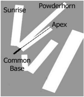
As width of the white bars is scaled to 100 feet per 300 p/h, a double chair would typically measure 400', a triple 600' and a quad 800' across the fall line. For areas that measure less than 30% slope, up to twice as many people can be assigned to the width when trails are covered by snowmaking and are regularly groomed. Good spacing of lifts prevents overlapping of (white) bars.
